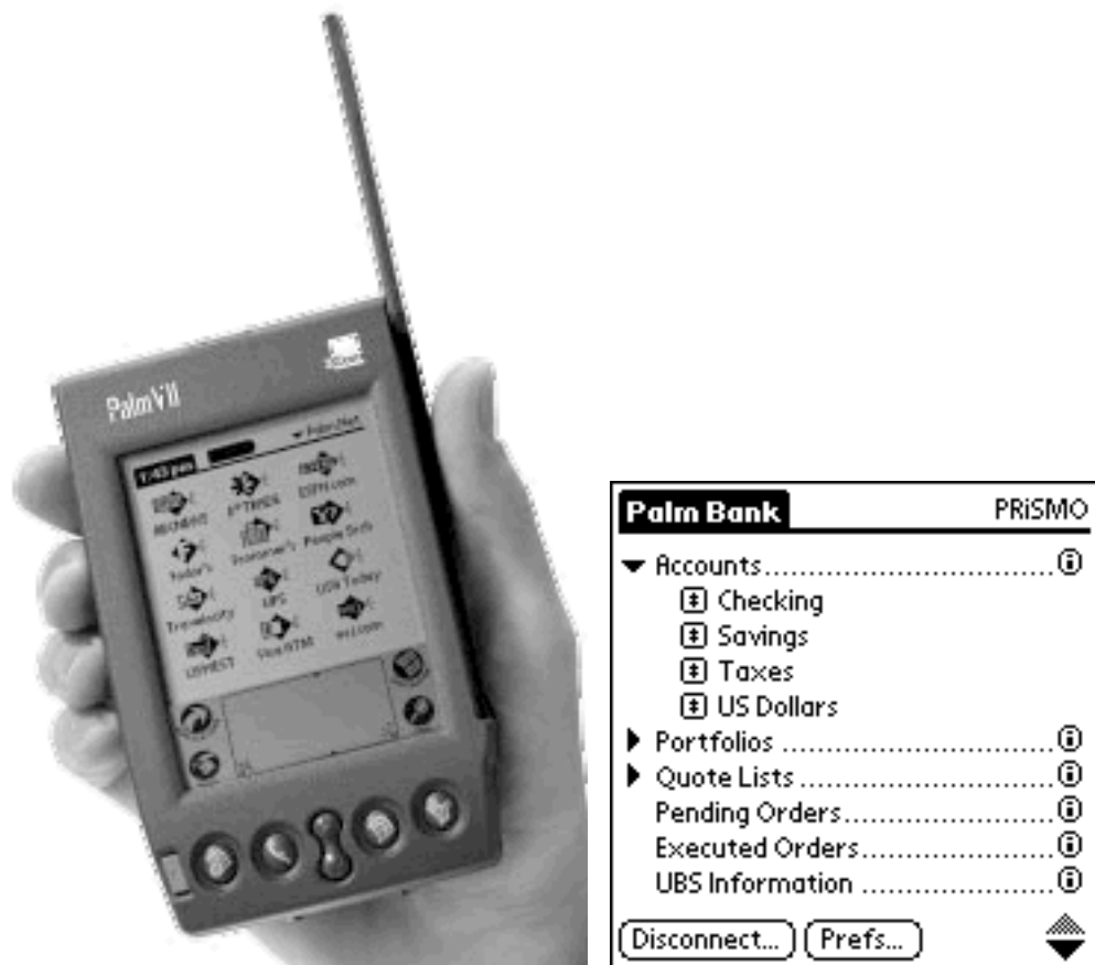
Figure 0.2 Palm VII with wireless Internet access and innovative main page with tree view
